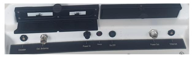
${\it Photo 4: Connector panel with battery compartment one lid open. External Antenna connector for GPS antenna.}$
