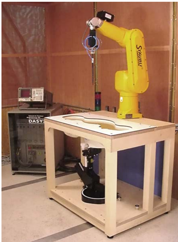
DASY3 SAR Measurement System with SAM phantom
