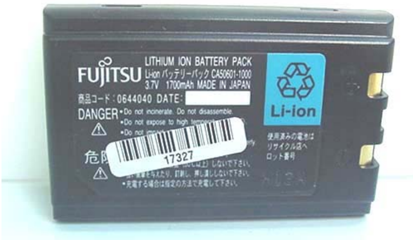
3.7 V 1700 mAh Li-ion Battery Pack
