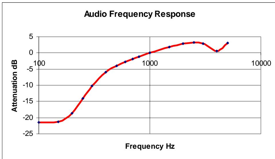
2.1047(b) Audio input versus modulation
