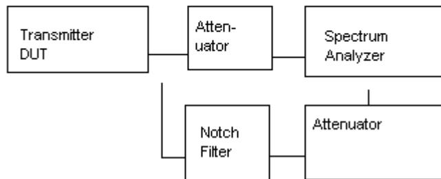
Method of Measuring Conducted Spurious Emissions
