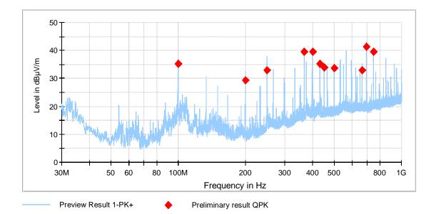
The following frequencies were found emission test outside restricted bands during the preliminary radiated:
