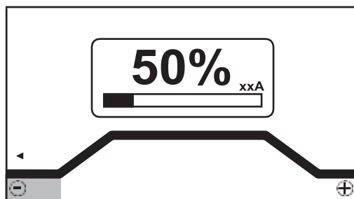
Starting current, 2-step mode and spot welding
