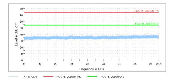
Spurious emissions from 18 – 26.5 GHz (Operation mode 2; Preliminary plot): no significant emission, no final measurement
