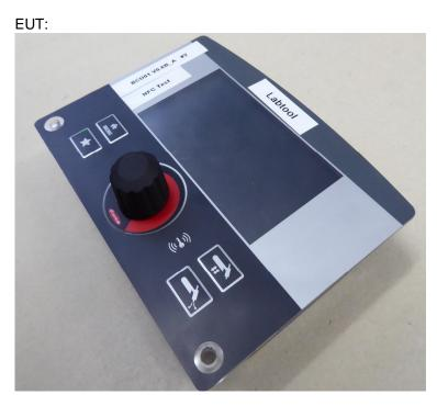
As declared by the applicant, only the 13.56.MHz RFID, Bluetooth low energy and Wi-Fi (2.4 GHz) will be used in the final application.
