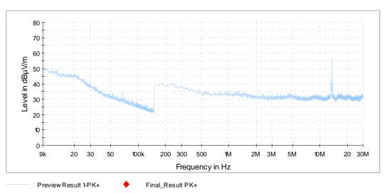
The emission at 68 kHz is caused by the measuring system and is therefore not measured. The emission at 13.56 MHz is a wanted signal and is therefore not rated, in this test report.
