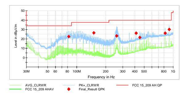
The following frequencies were found emission test outside restricted bands during the preliminary radiated:
