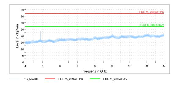
170756 12-18GHz ch19: Spurious emissions from 12 GHz to 18 GHz (operation mode 2):
