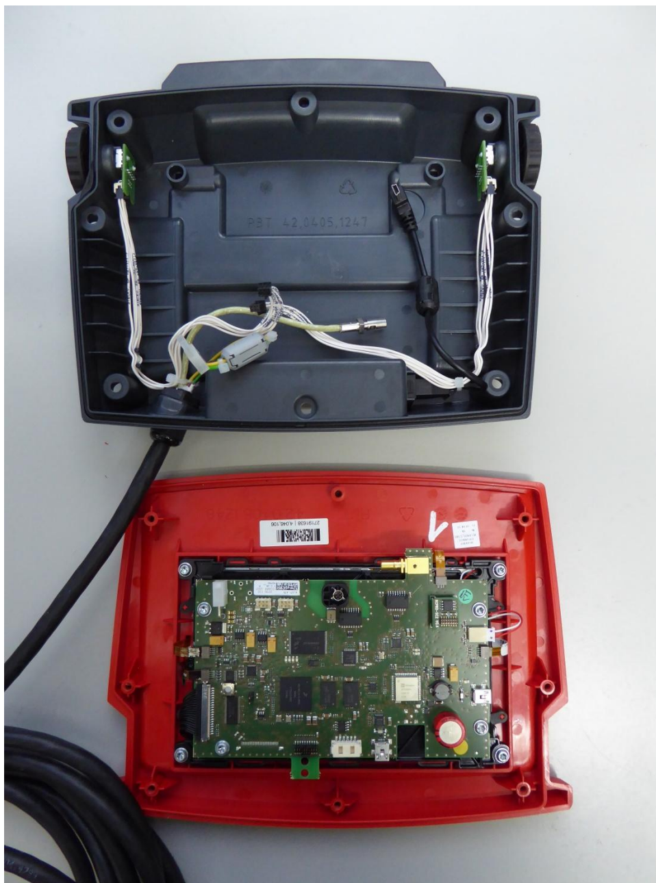
161548_10.JPG: RC Panel Pro, internal view 1
