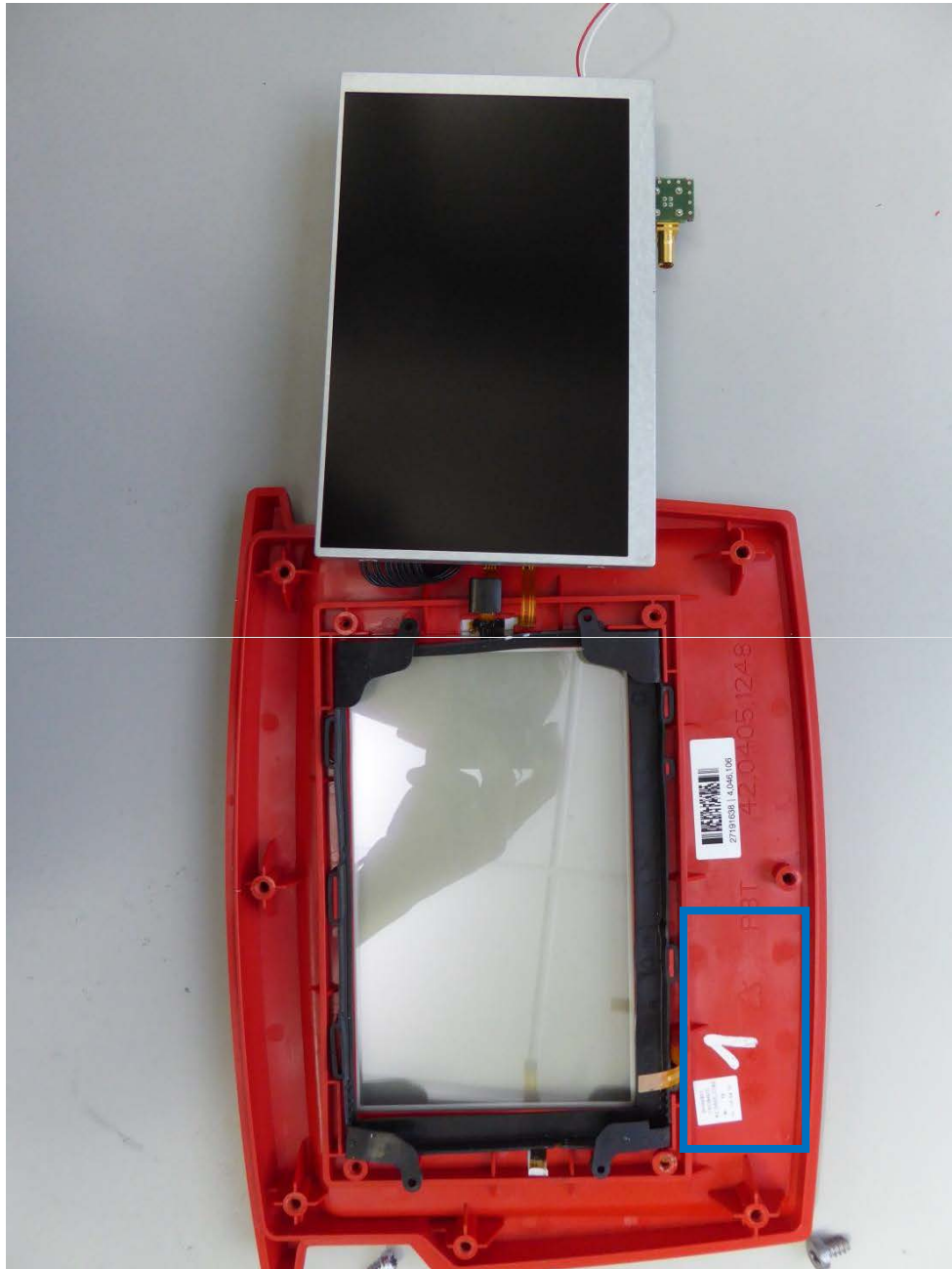
161548_14.JPG: RC Panel Pro, internal view 5 The blue square indicates the antenna location.
