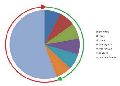
The module stays infinitely in this loop until a reset from the user is received or a target is detected (placed into the field). A target can be a RFID transponder card (e.g. Mifare) or an NFC enabled device (not part of the EUT).
