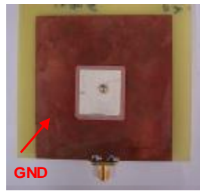
Figure 13 GPS demo board
