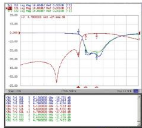
2012 / 5GHz WLAN Low Pass Filter CFL4111 714505004K
