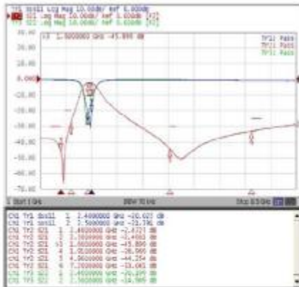
1608 / 2.45GHz Bluetooth /WLAN Band Pass Filter CFL4111715012454K
