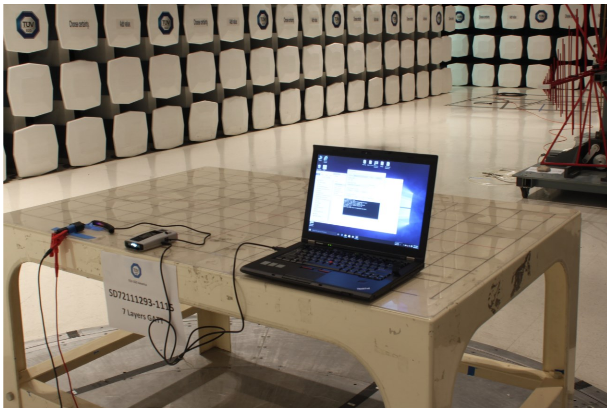
Radiated Emissions Test Setup installed in a host (below 1GHz in test mode)
