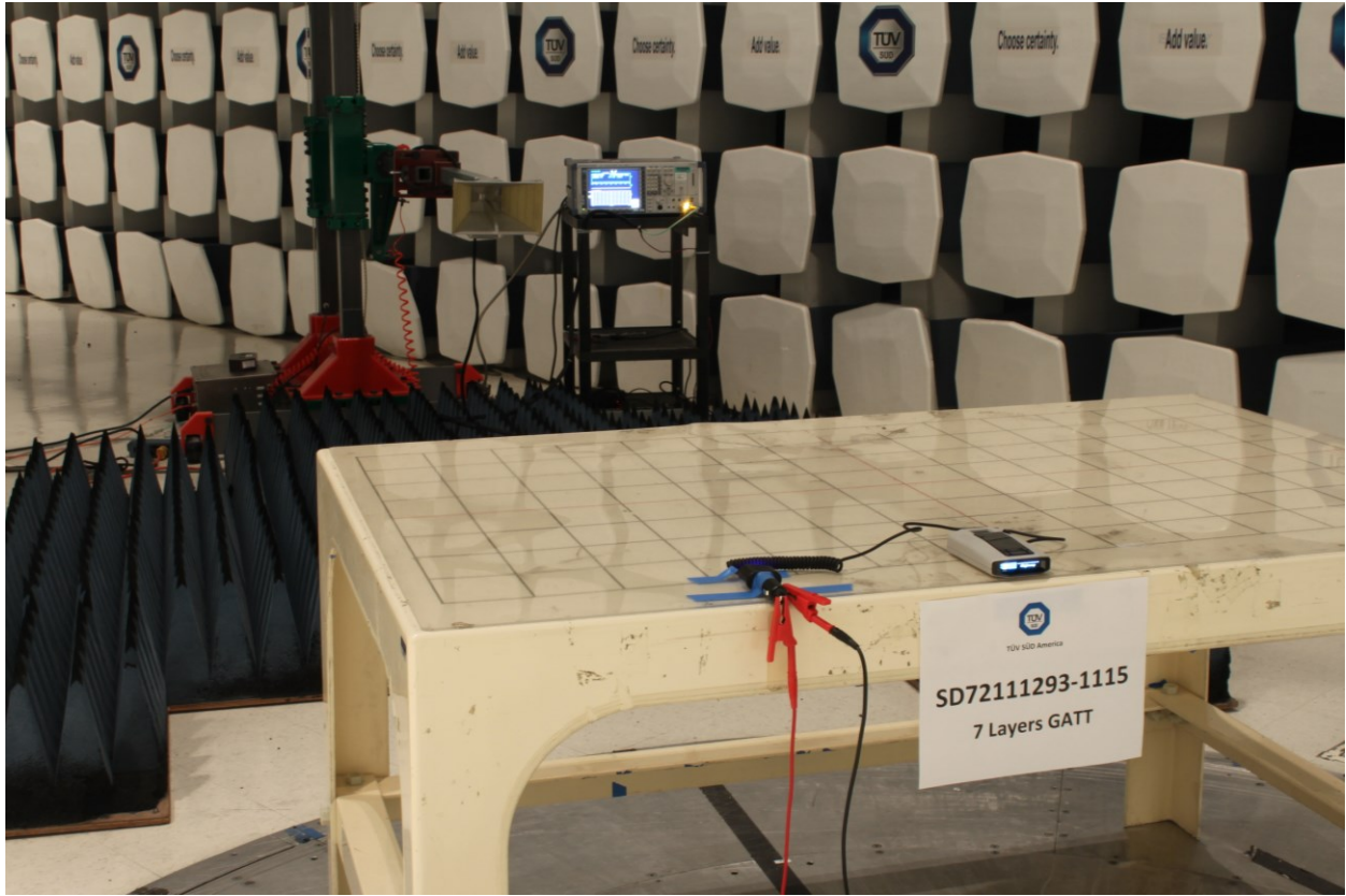
Radiated Emissions Test Setup installed in a host (above 1GHz in normal mode)
