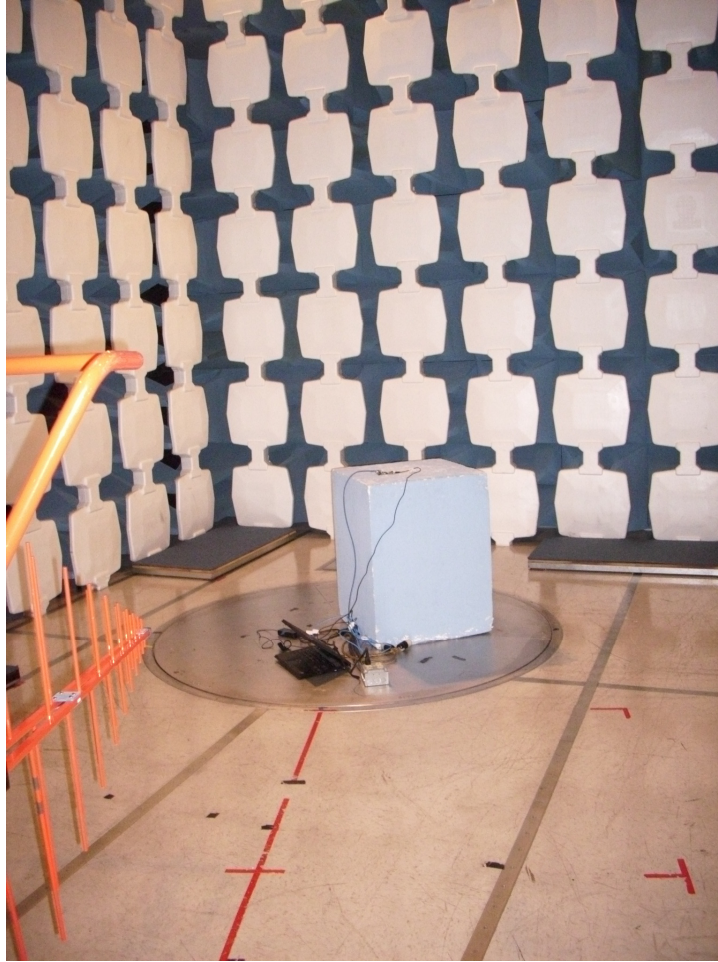
Radiated Emissions Measurements – Below 1GHz – Anechoic Chamber
