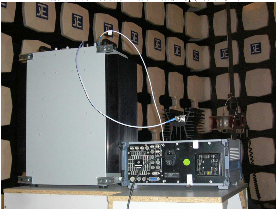
Measurement of Radiated Emission Test Set Up (Above 1GHz)
