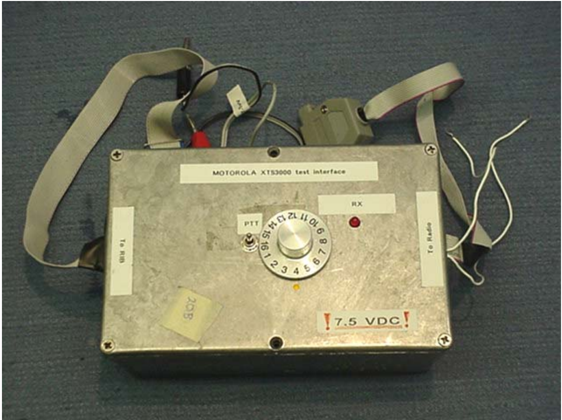
Test interface box
