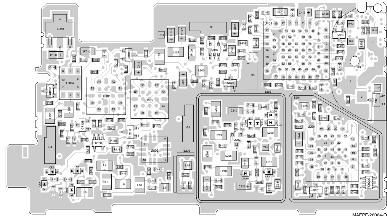
NLE4249A UHF Range 1 RF Board Component Location Detail and Parts List
