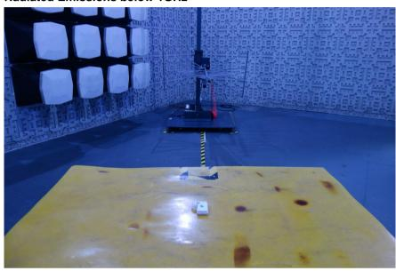
Field Strength of the Fundamental Signal (15.231(b))
