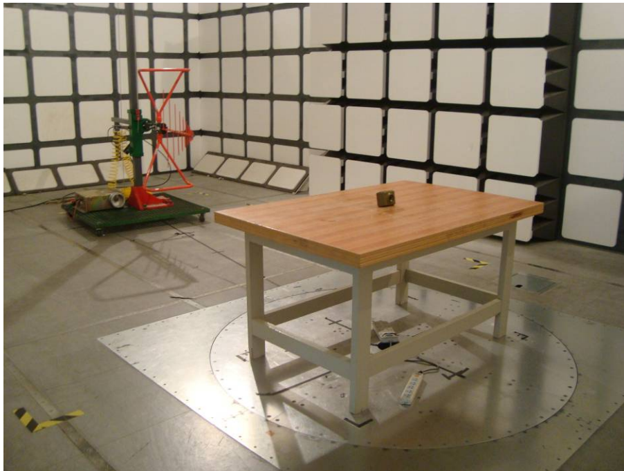
Radiated Emission – Front View (Below 1GHz)
