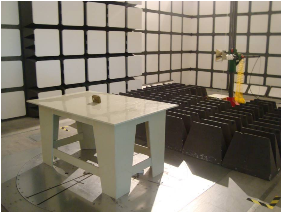
Radiated Emission – Rear View (Above 1GHz)
