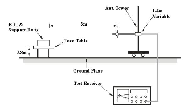
The radiated emission tests were performed in the 3-meter Chamber, using the setup accordance with the ANSI C63.4 - 2003. The specification used was the FCC 15 § 15.231(b)"
