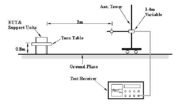
The deactivation test was performed in the 3-meter Chamber, using the setup accordance with the ANSI C63.4 - 2003. The specification used was the FCC 15.231(a) limits.
