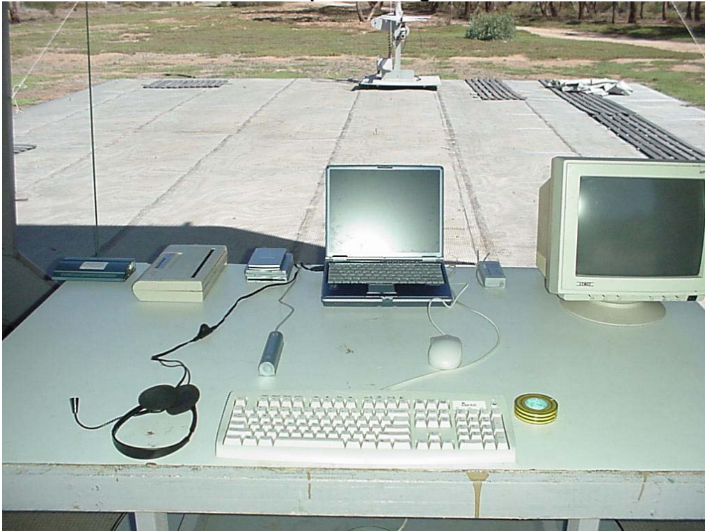
Radiated Emissions Test Set Up - Host 'Ginger' Lifebook
