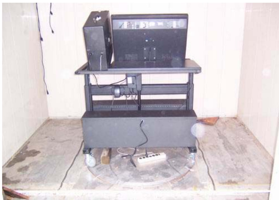
Figure 3.2 Radiated Test Setup -Back
