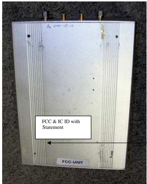
Figure 2 Proposed FCC/IC ID Label Location on U-3000
