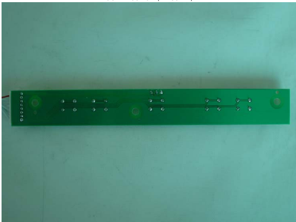
OSD Board ( Rear )
