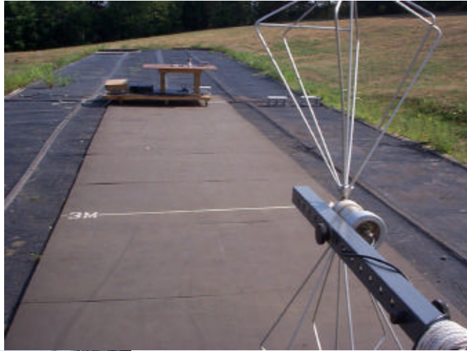
Biconical antenna Frequency range 30-200MHz
