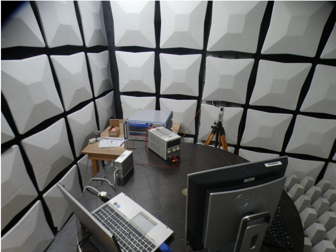
Photo 13: Test setup for radiated measurements, FCC Part 15 subpart B, ICES 003 and CISPR 22, between 26 GHz and 40 GHz
