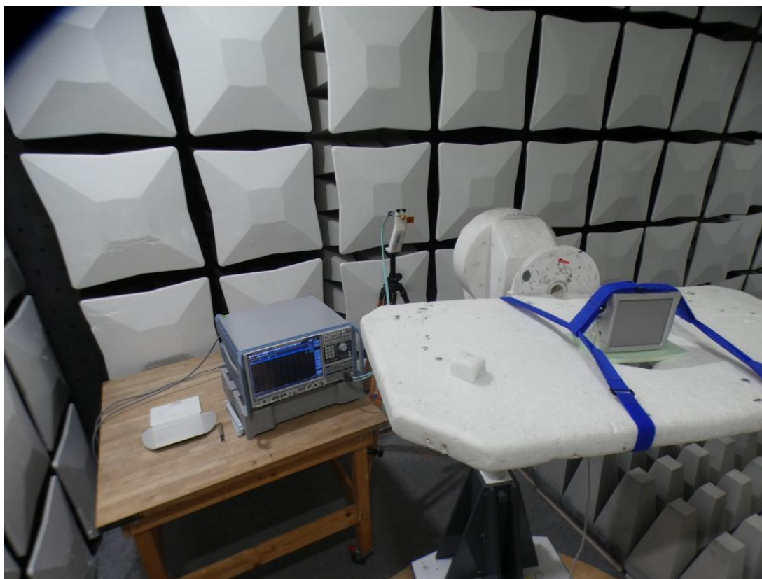
Photo 7: Test setup for radiated measurements, between 60 GHz and 90 GHz
