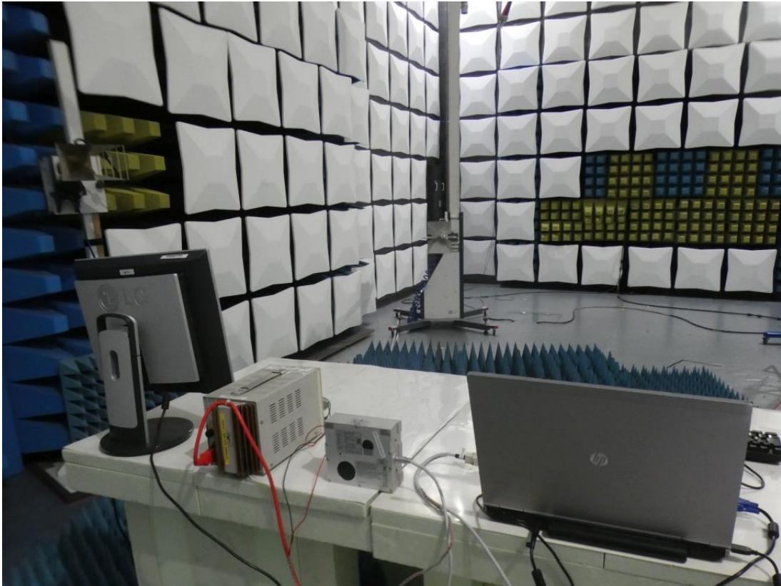
Photo 11: Test setup for radiated measurements, FCC Part 15 subpart B, ICES 003 and CISPR 22, between 1 GHz and 18 GHz
