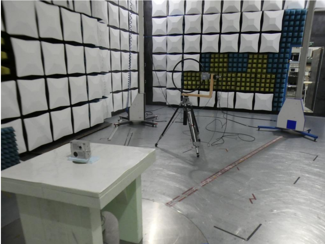
Photo 1: Test setup for radiated measurements, under 30 MHz
