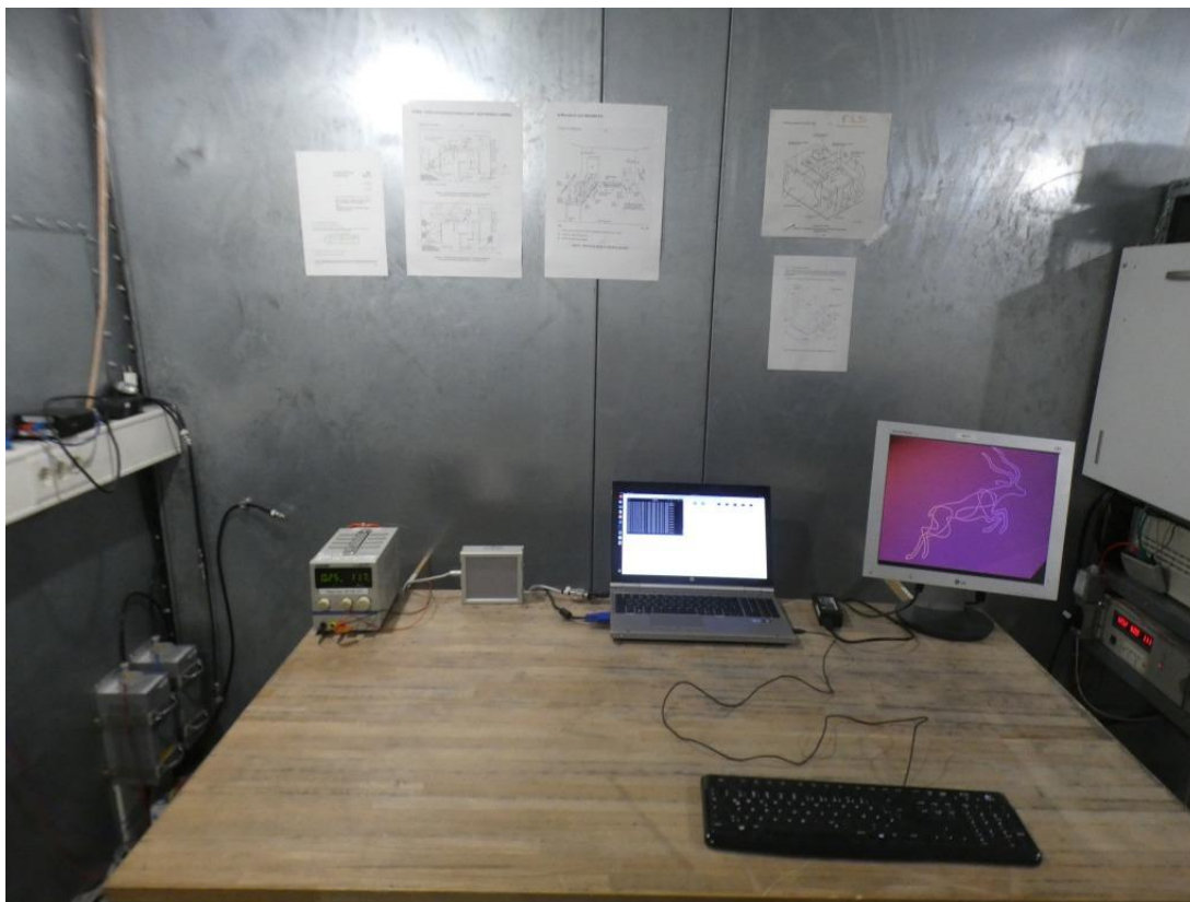
Photo 9: Test setup for conducted measurements, FCC Part 15 subpart B, ICES 003 and CISPR 22
