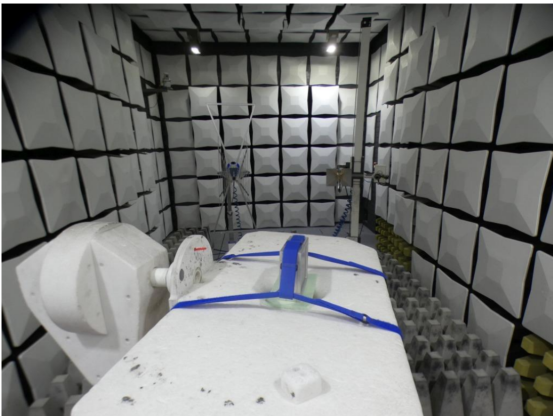
Photo 4: Test setup for radiated measurements, between 18 GHz and 26 GHz
