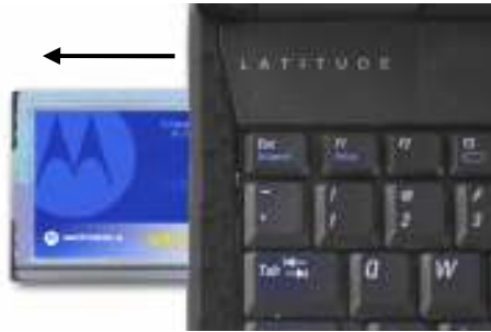
Figure 3-19 Removing the WMC6300 from the PCMCIA slot
