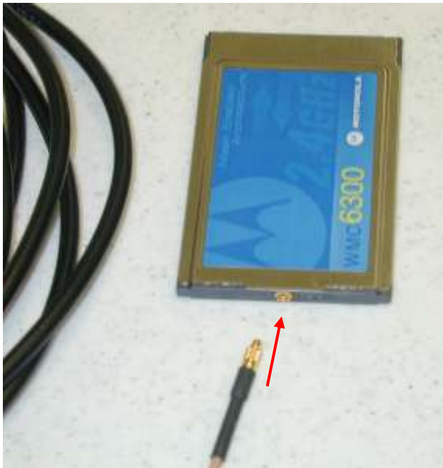
Figure 3-4 N-Type SMA to the MMCX adapter connecting to the WMC6300
