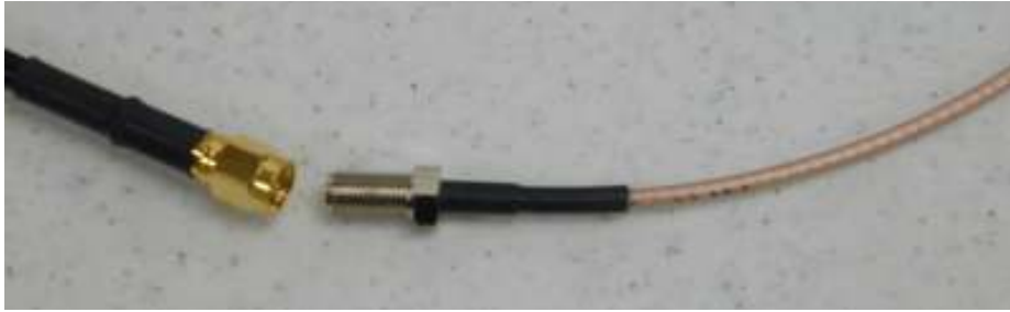
Figure 3-3 Antenna Cable end connecting to MMCX adapter
