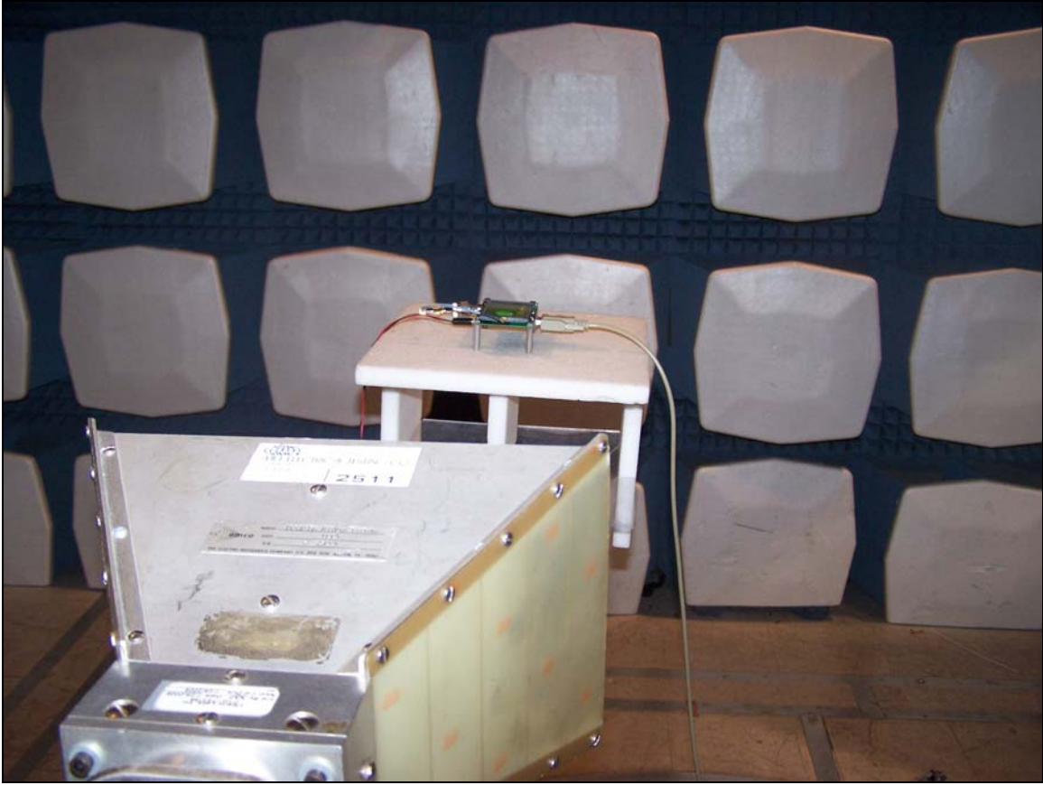
Photograph 2. Radiated Emissions, Test Setup
