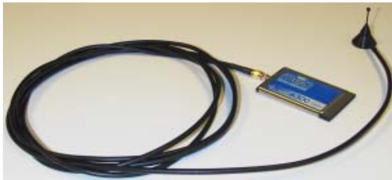
Figure 14. Attach Magnetic Mount Antenna to the WMC6300
