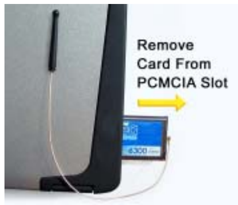
Figure 18. Removing the WMC6300 from the PCMCIA slot
