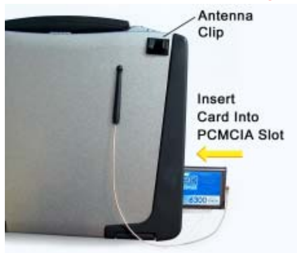
Figure 12. Mounting the Antenna Clip
