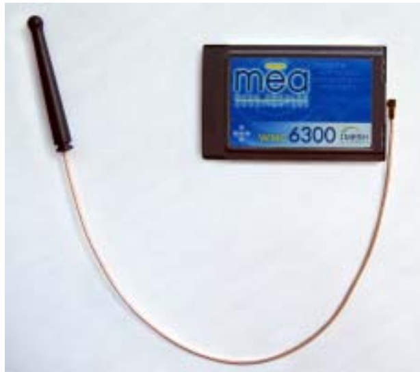
Figure 10. Attach Antenna to the WMC6300
