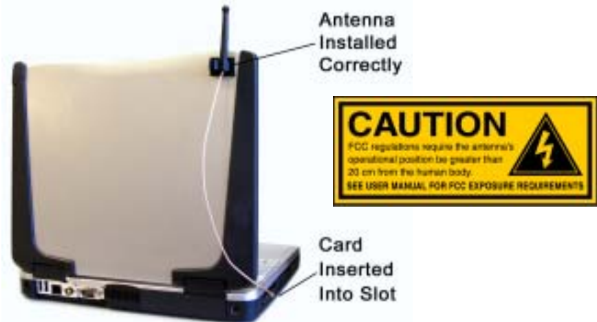
Figure 13. Insert the Antenna into the Clip
