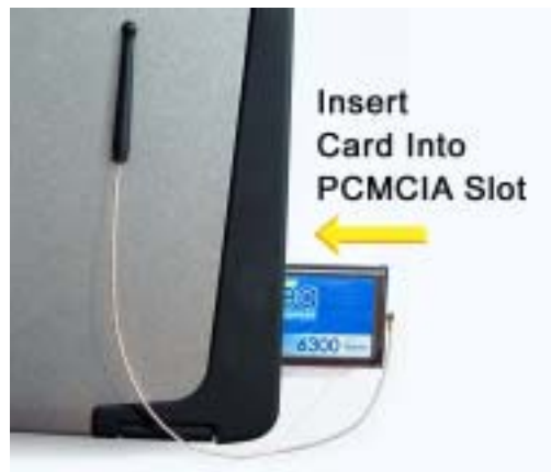
Figure 15. Installing the WMC6300 Wireless Modem Card
