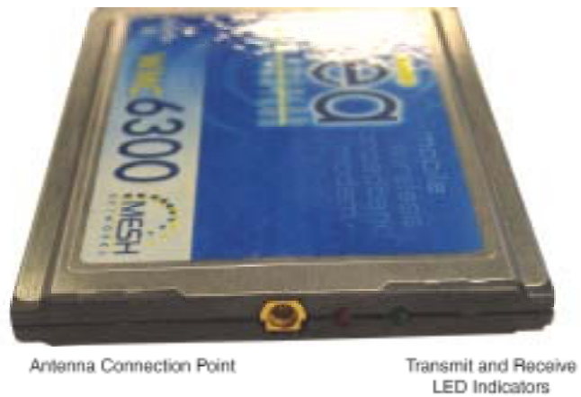
Figure 3. WMC6300 Antenna Port and LED Indicators
