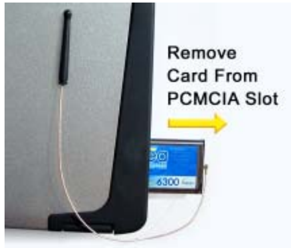
Figure 18. Removing the WMC6300 from the PCMCIA slot
