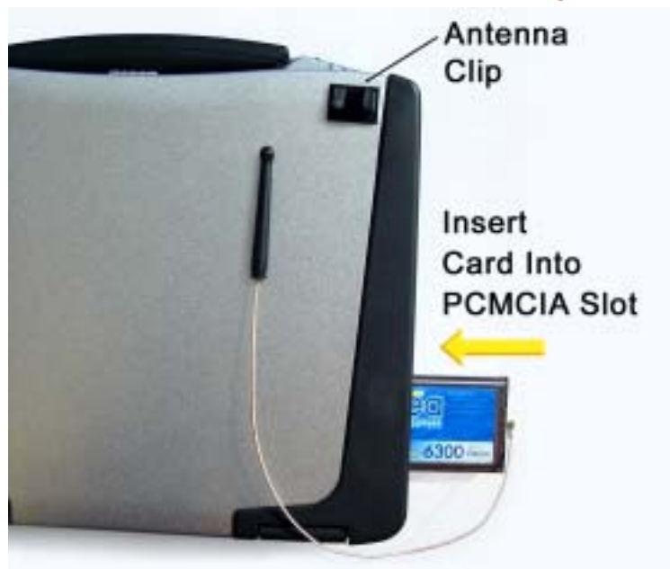
Figure 13. Mounting the Antenna Clip
