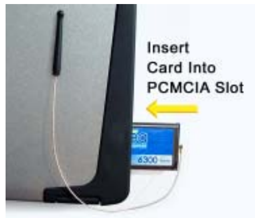
Figure 16. Installing the WMC6300 Wireless Modem Card
