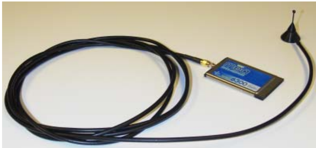
Figure 15. Attach Magnetic Mount Antenna to the WMC6300
