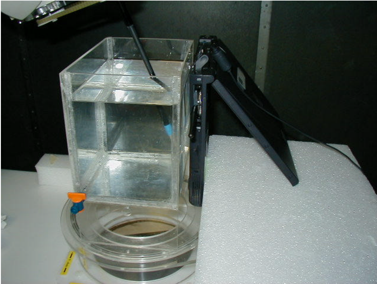
Figure S11. Setup Configuration 3 of table 10, 11 and 12 ( the EUT's bottom-face is in parallel and in contact (0 cm) with the flat phantom)
