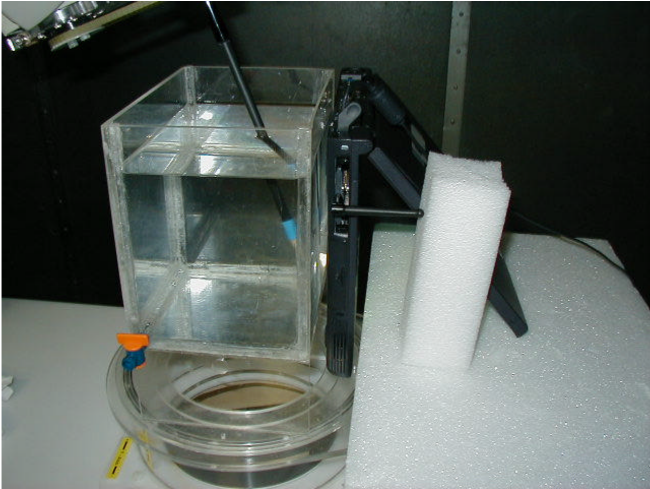
Figure S10. Setup Configuration 1 of table 10, 11 and 12 ( the EUT's bottom-face is in parallel and in contact (0 cm) with the flat phantom)
