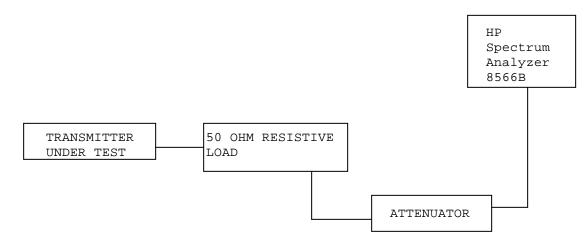
NAME OF TEST: SPURIOUS EMISSIONS AT ANTENNA TERMINALS
