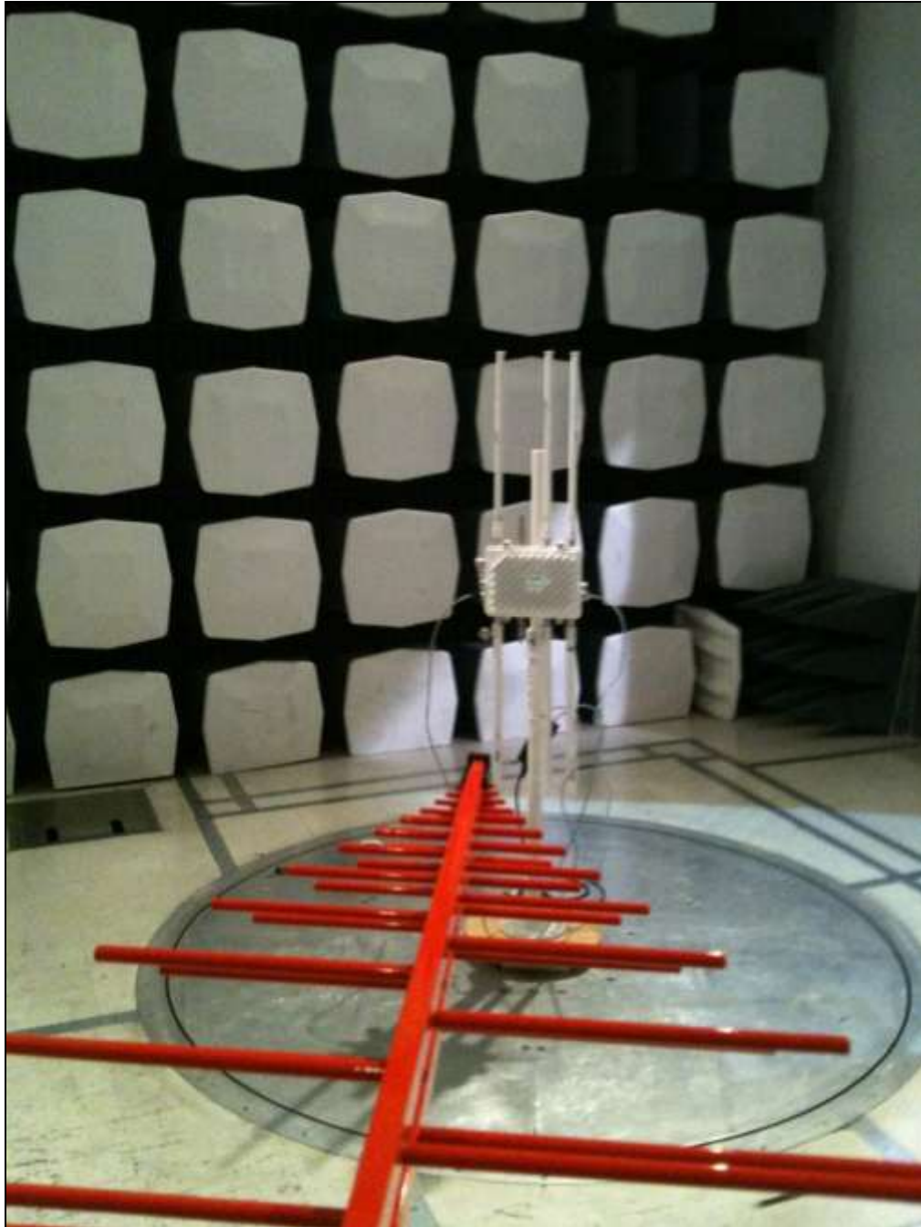
Photograph 3. Radiated Emission, Test Setup
