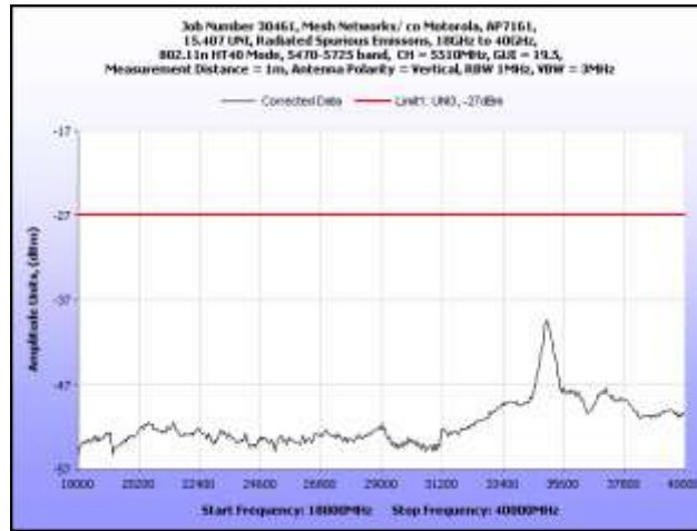
Plot 232. Radiated Spurious Emissions, 18 GHz – 40 GHz, 802.11n HT40, 5510 MHz
