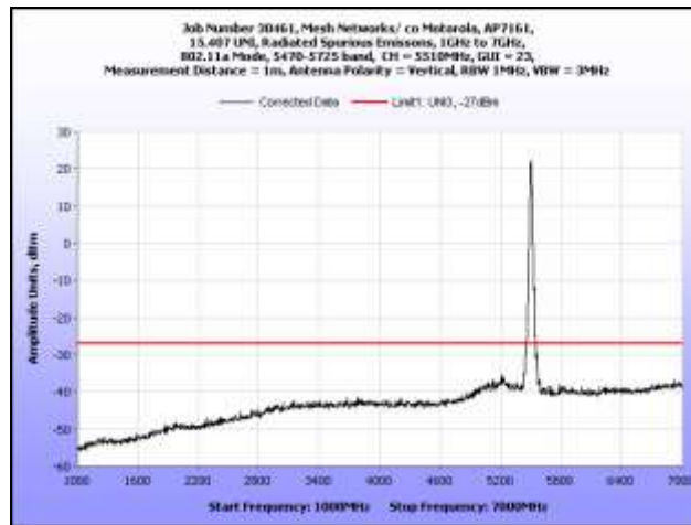
Plot 230. Radiated Spurious Emissions, 1 GHz – 7 GHz, 802.11n HT40, 5500 MHz
