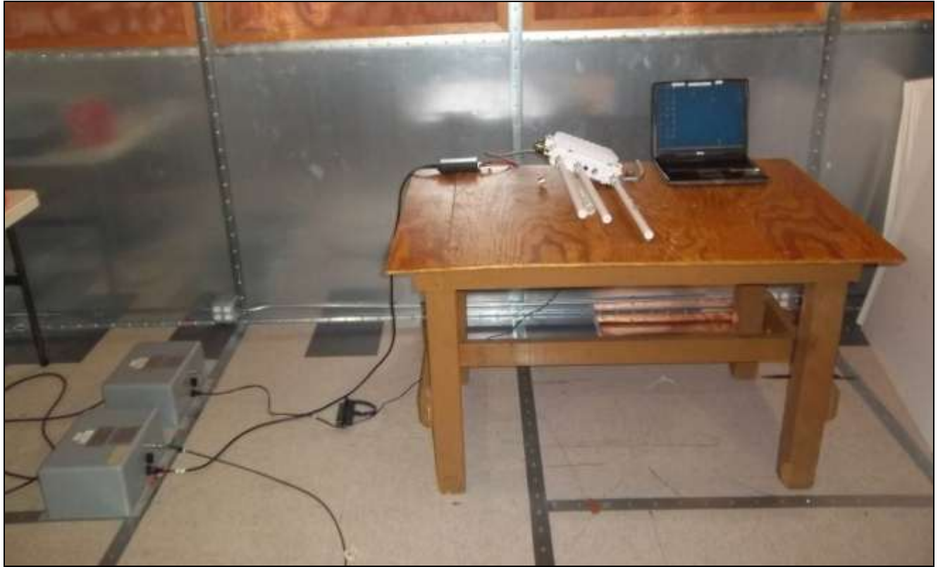
Photograph 2. Conducted Emissions, Test Setup
