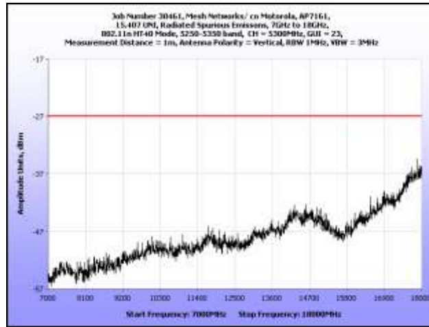
Plot 223. Radiated Spurious Emissions, 7 GHz – 18 GHz, 802.11n HT40, 5300 MHz
