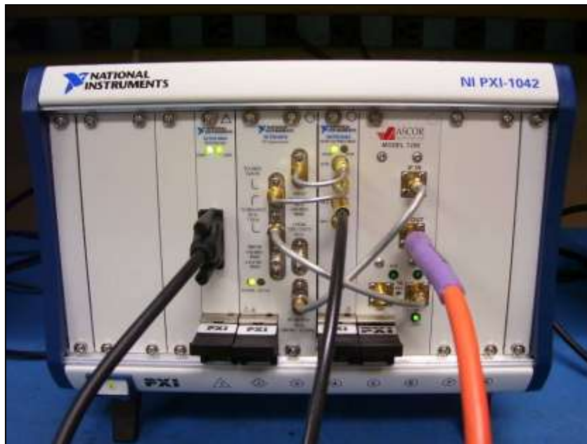
Photograph 8. DFS Radar Test Signal Generator
