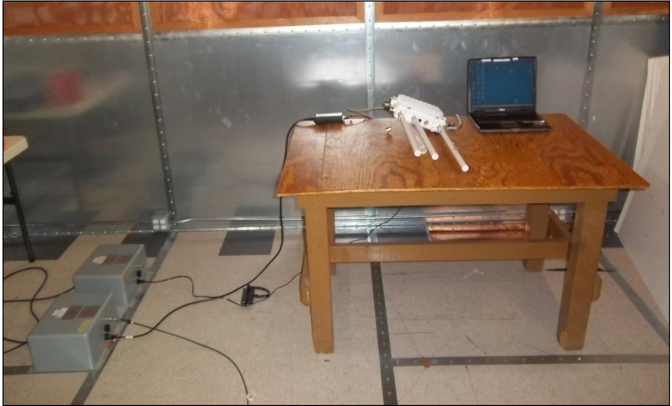
Photograph 4. Conducted Emissions (15.207) Test Setup PoE30U-560
