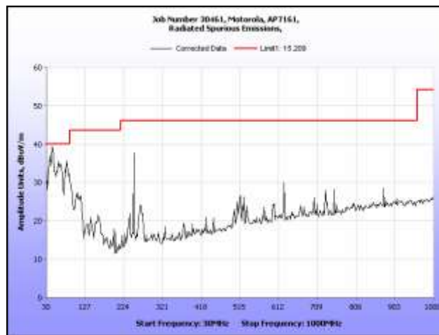
Plot 233. Radiated Spurious Emissions, 30 MHz – 1 GHz, 802.11n HT40, 5670 MHz
