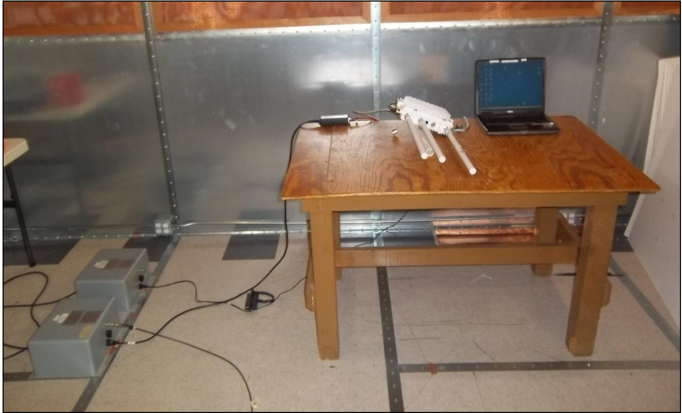
Photograph 4. Conducted Emissions (15.207) Test Setup PoE30U-560
