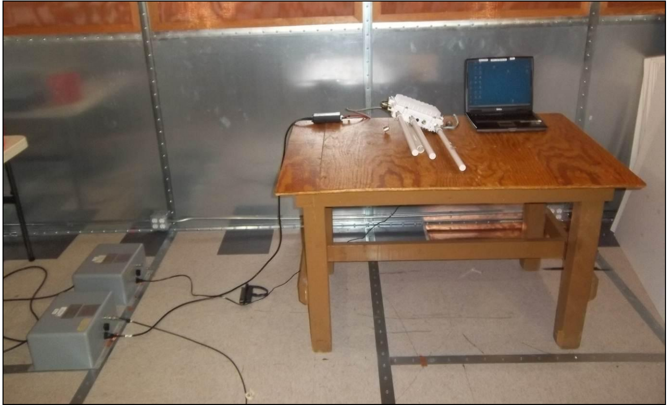
Photograph 2. Conducted Emissions, Test Setup
