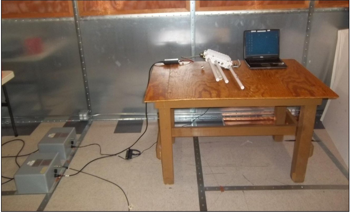
Photograph 3. Conducted Emissions (15.207) Test Setup PoE30U-560
