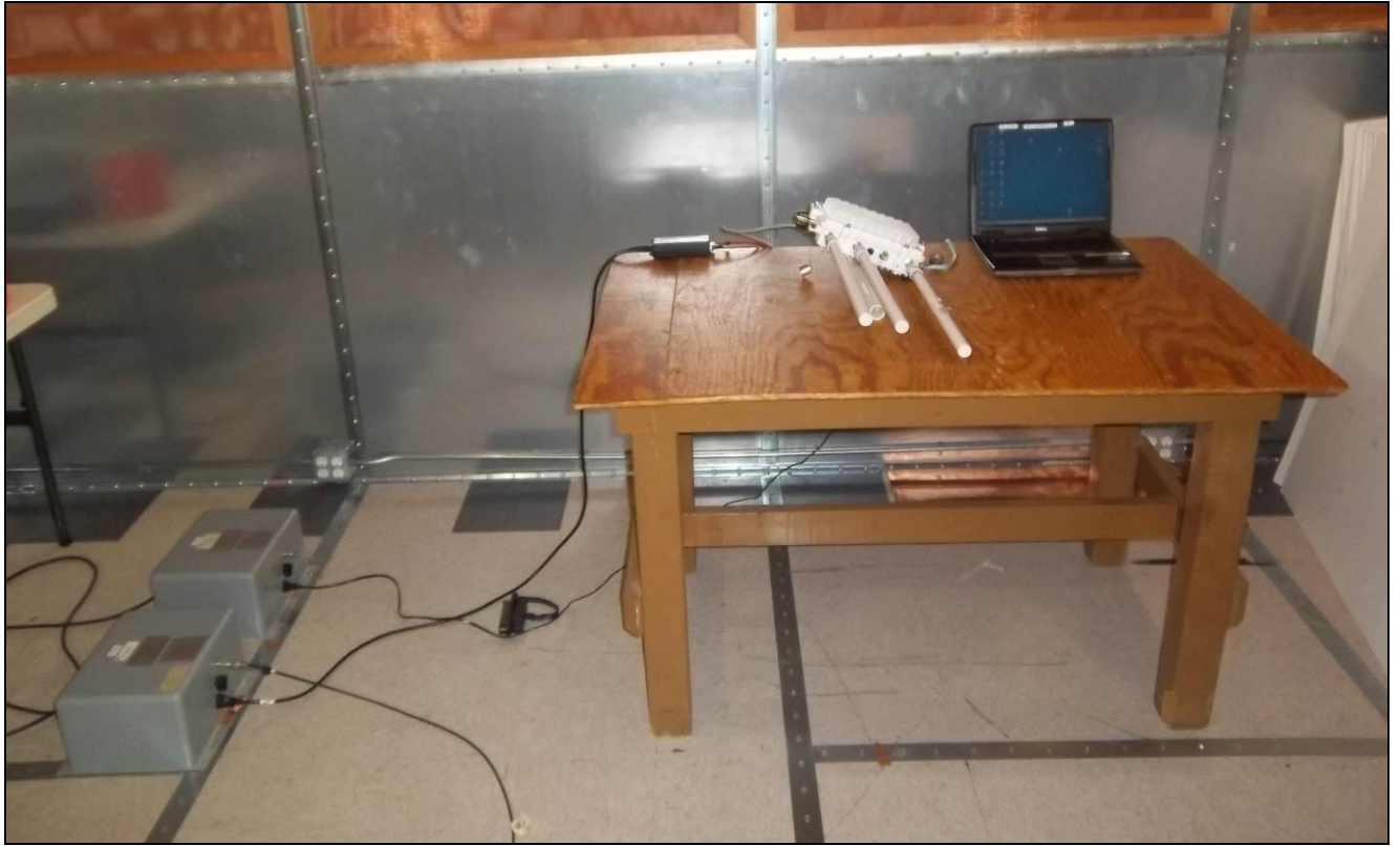
Photograph 1. Conducted Emissions, Test Setup
