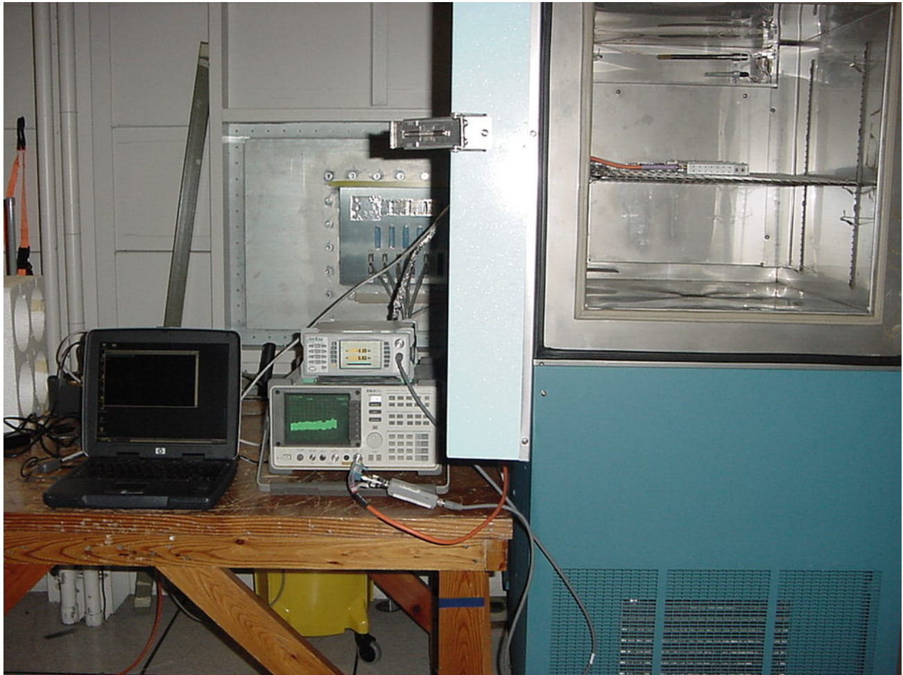
Photograph 6. Frequency Stability Test Setup
