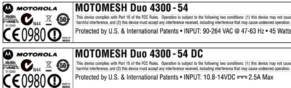
Figure 2-4 MOTOMESH DUO 4300 - 54 AC and DC Device Product Label (Samples for European Use only)
