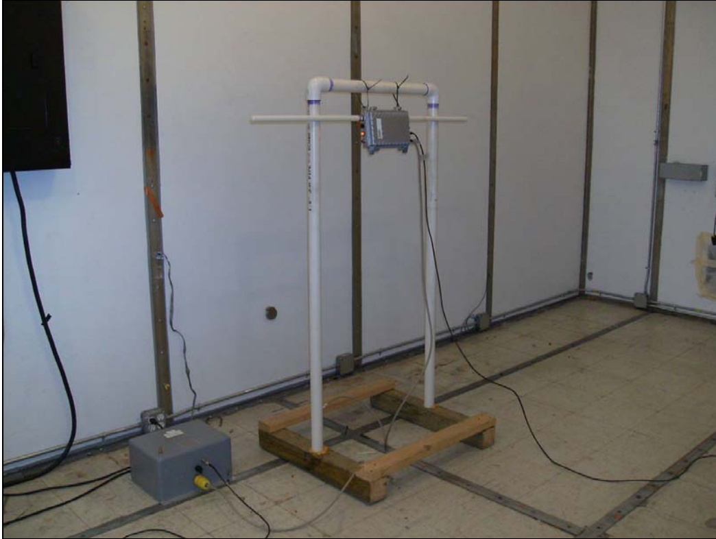
Photograph 2. Conducted Emission Test Setup
