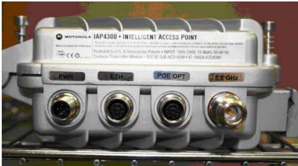
Figure 2-6 Close Up of External Connection Points
