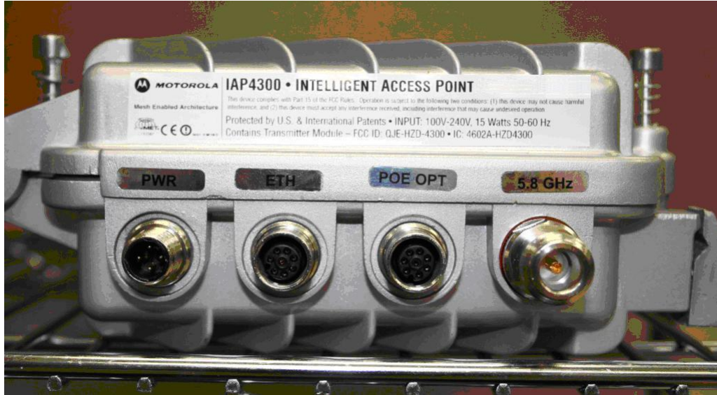
Figure 2-6 Close Up of External Connection Points
