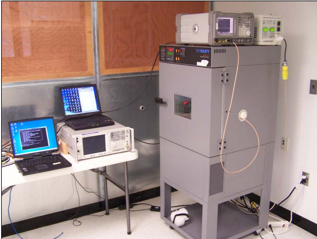
Photograph 5. Frequency Stability Test Setup
