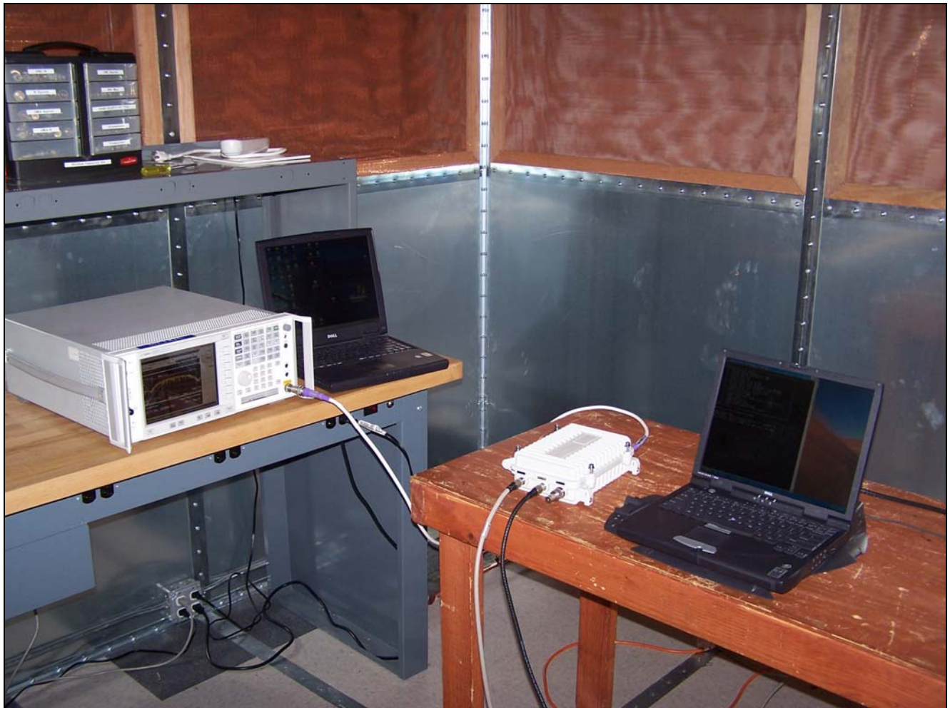
Photograph 4. Peak Power Output and RF Exposure, Test Setup
