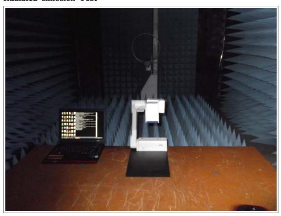
Radiated emission Test
