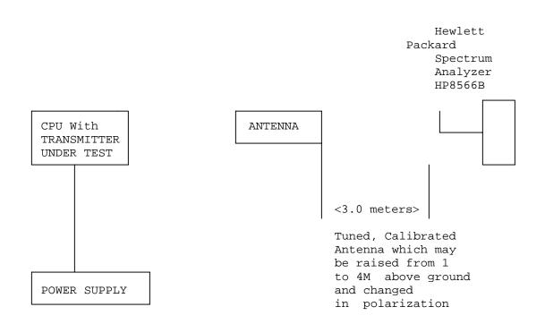
Equipment placed 80cm above ground on a rotatable platform.
