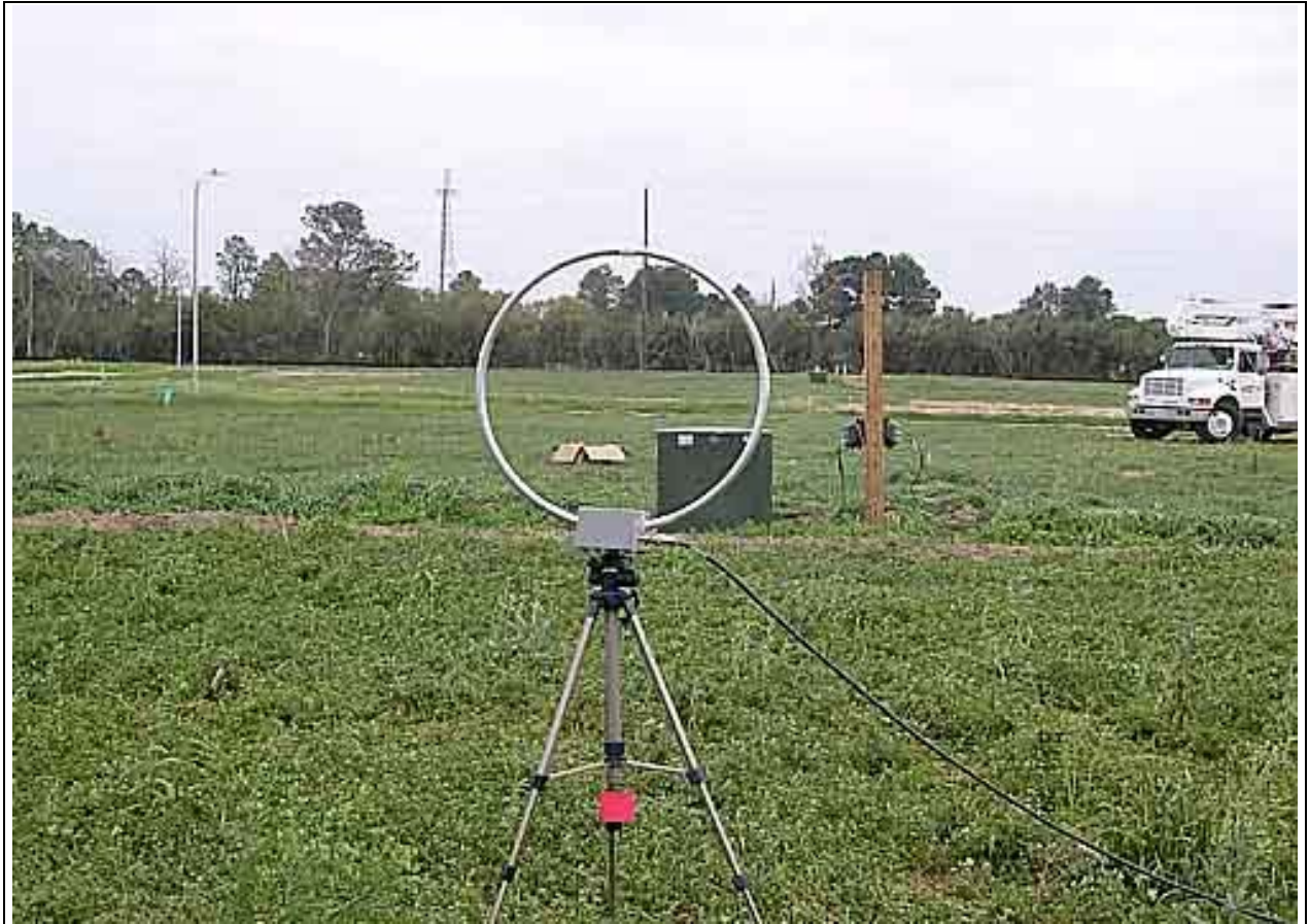
Position 5, 20-30 MHz Parallel (behind transformer)
