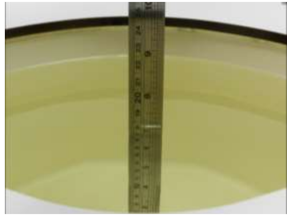
Fig 10.2 Photo of Liquid Height for Body SAR
