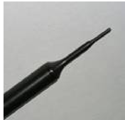
Figure 2. EX3DV4 E-field Probe
