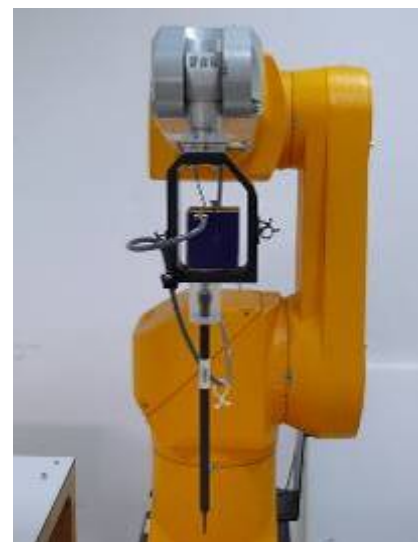
Figure 3. EX3DV4 E-field probe
