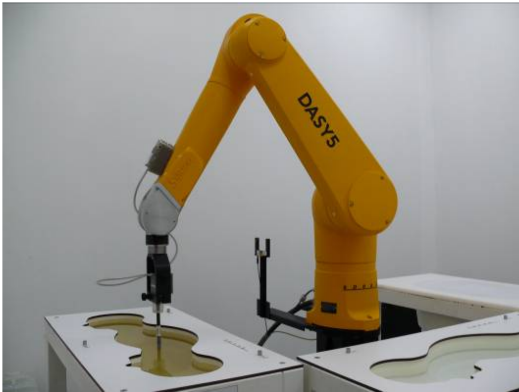
Picture 1: Specific Absorption Rate Test Layout
